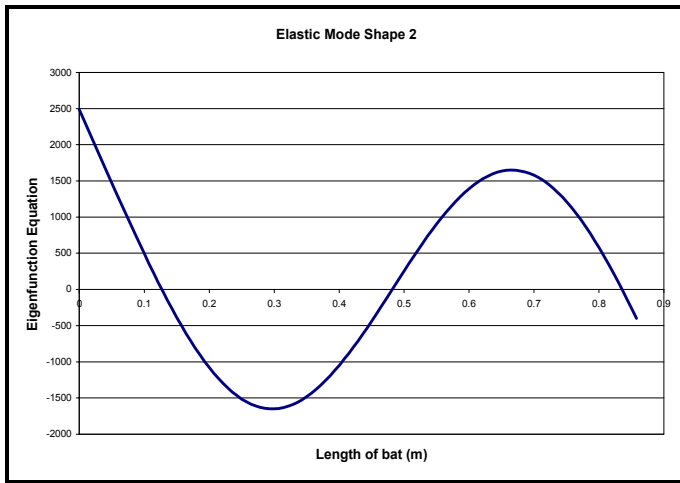
Figure 15. 1 st Elastic Mode Shape of Beam Equation
